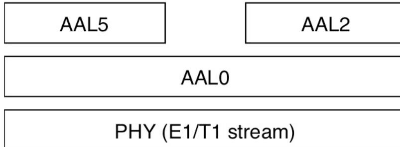
Monitoring at the AAL0, AAL2 and AAL5 interfaces is supported. The monitored information is extracted, filtered and sent via TCP/IP to an application host. Statistics are gathered.
